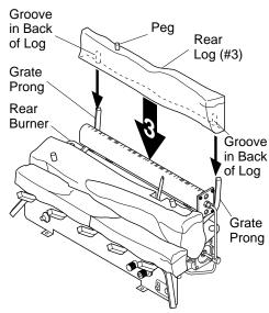
Figure 18 - Installing Rear Log (#3)
